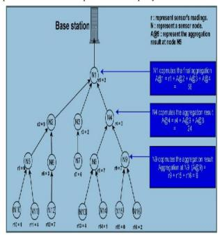
Figure 2: Secure Data Aggregation
